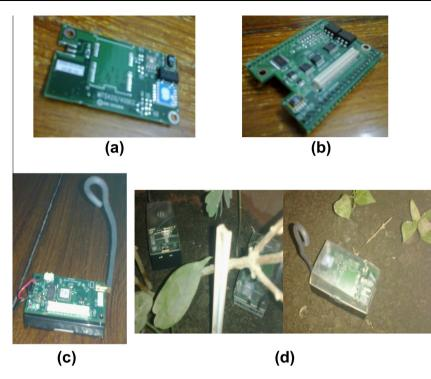
Figure 3 Sensor nodes hardware and deployment.
