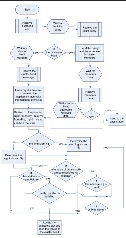
Figure 9 Sensor node procedures.
