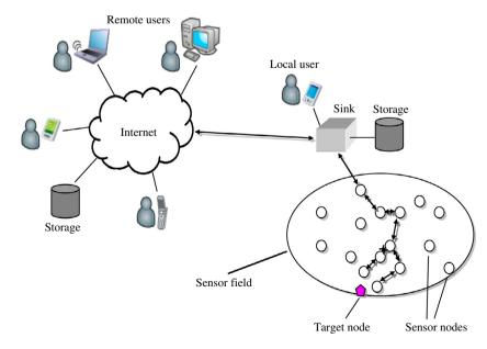
Figure 2 Sensor nodes scattered in a sensor field [6].
