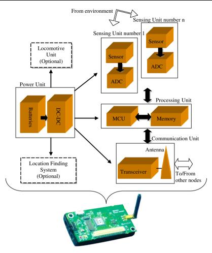
Figure 1 The components of a sensor node [6].
