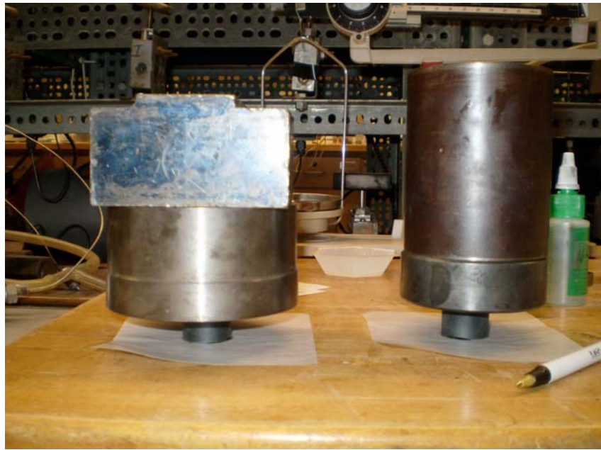
Figure 10. Post-run graphite capsules were placed in a sample holder and set in epoxy resin. Weights were used to keep the epoxy within the holder as it hardened.
