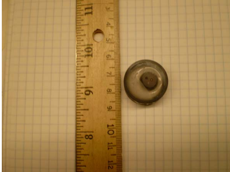
Figure 11. Image of a sample polished, carbon coated, and ready to go into the SEM for analysis. Actually sample mixtures are the 2 mm diameter darker spots within the graphite capsule.
