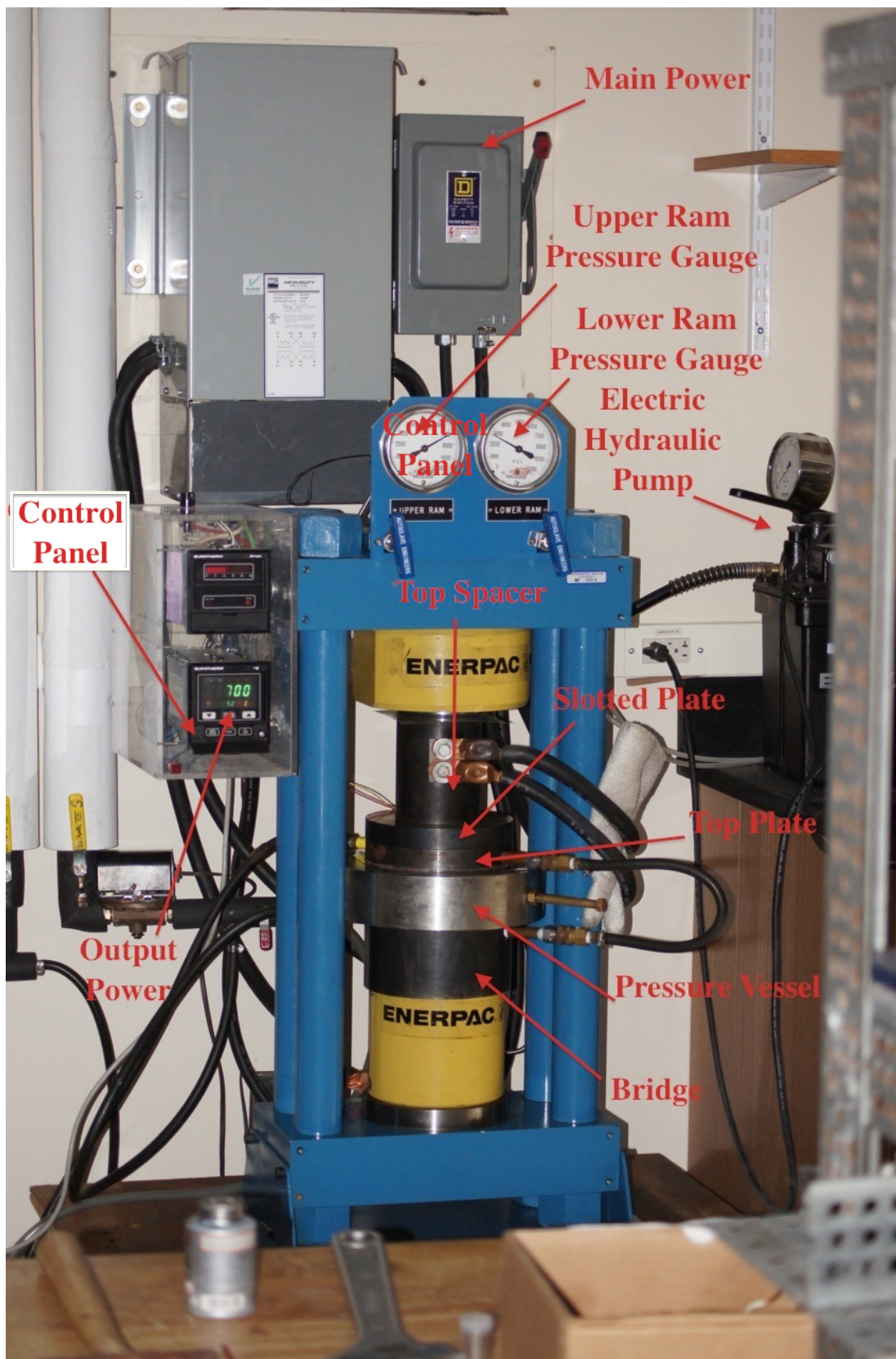
Figure 3: Photograph of piston cylinder press during the 700°C run. Main components of the press are labeled in red. Parts not seen in this image are the thermocouple assembly, the carbide pusher, piston, donut and spacer. Recirculating water hoses connect the bridge and the top plate.
