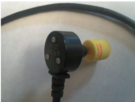
Figure 1: ER-10C probe marked for different positions using electronic caliper
