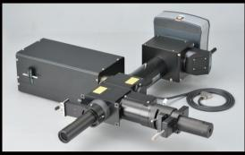
Motorized main branch + motorized sub branch + H-TIRF module + DMD module + LED adapter + EPI FL module
