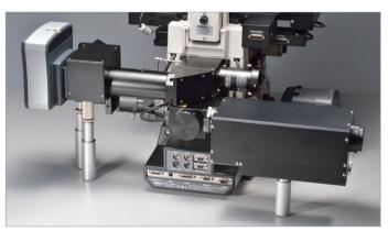
Example: A DMD module (upper tier), H-TIRF module and EPI FL module (lower tier) are attached.
