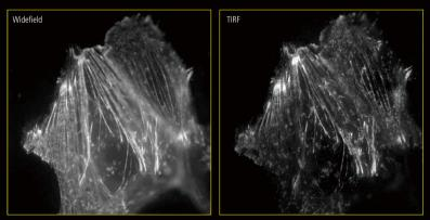
A cell expressing GFP-tagged actin was imaged using the epi-fluorescence illuminator (left panel) and the H-TIRF illuminator (right panel).
