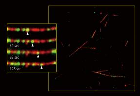
An in vitro preparation of fluorescently-labeled microtubules (Alexa 647) and dynein (tetramethylrhodamine) was imaged as a time series using the H-TIRF illuminator. Single molecules of dynein (in green) can be visualized moving along microtubules shown in red (see insert for a time series of one of the microtubules at a higher magnification; arrowheads point to a moving dynein molecule).
