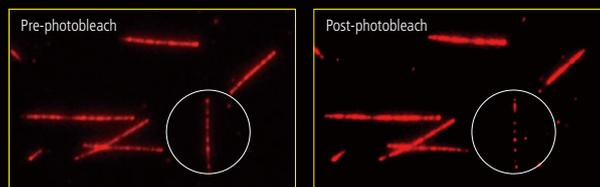
*An in vitro* preparation of fluorescently-labeled microtubules (Alexa 488) and dynein (tetramethylrhodamine) was imaged using the H-TIRF illuminator. This preparation contained high concentrations of dynein and single motor molecules were difficult to visualize. By using the FRAP module to photobleach a large portion of the motor molecules bound to a microtubule, single molecules of dynein could be clearly visualized (compare pre- and post-photobleach panels; photobleached area is circled).
