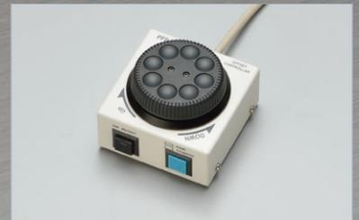
Real-time offset amount of Z-axis depth can be controlled after PFS setting.
