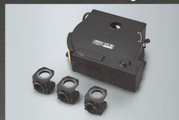
Position of fluorescence filter cubes can be changed in 0.3 sec. per position. (Photo shows high-performance type)
