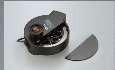
Fluorescence excitation filters (8 positions—using 25mm filters) can be changed at a high speed of 0.15 sec. between adjacent positions.
