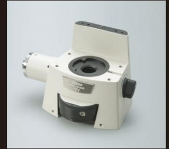
High-resolution imaging with "full intensity" external phase contrast system is possible. TV port is incorporated.
