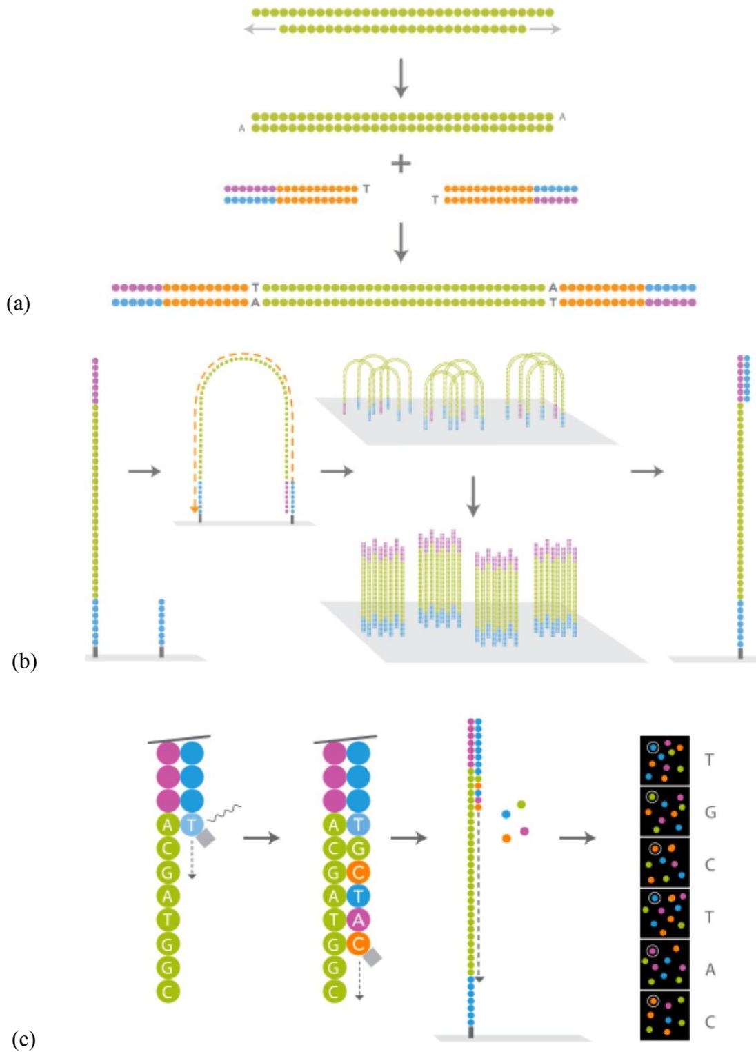
**Figure 4.** Illumina sequencing technology (a) Sample library preparation (b) Cluster generation (c) Sequencing-by-synthesis technology ([Illumina Sequencing Technology](#)) (Illumina, Inc<sup>®</sup>, 2012).
