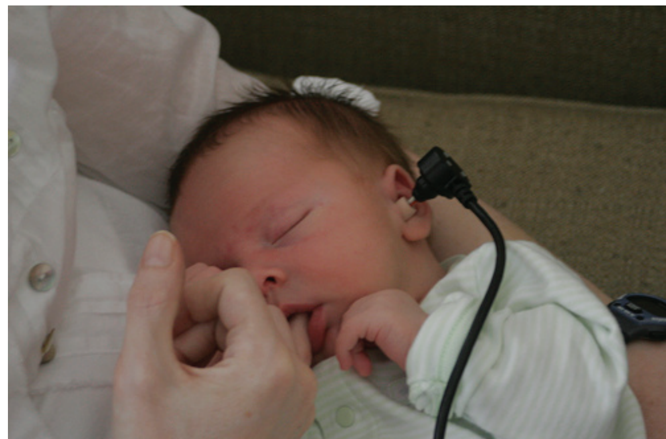
Figure 1: Reflectance measurement being made on an infant ear using an Etymotic ER-10c probe with 14B foam tip. (Photo used with permission from Navid Shahnaz.)
