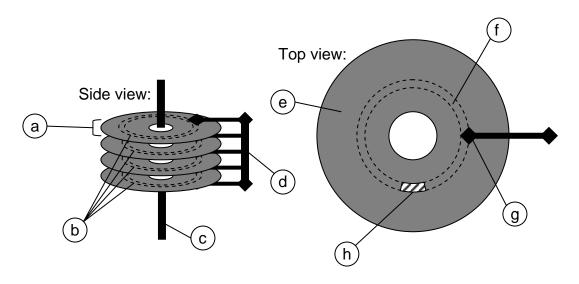
a = platter, b = cylinder, c = spindle, d = comb, e = surface, f = track, g = read/write head, h = sector.
