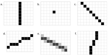
Algorithms: (I.) simple midpoint algorithm, (II.) iterative midpoint algorithm, (III.) Wu's antialiased line.
