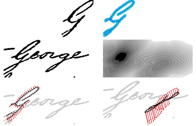
Figure 1. Several steps in the model fitting process. First row: a character G prototype and the corresponding model. Second row: a sample word and the corresponding fit score \mathcal{E}(\vec{v}) for the model G. Third row: recovered configurations for two local optima, with warping from the default configuration shown in red.
