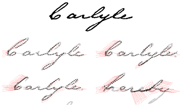
Fig. 5. Sample GW20 retrievals for singleton query word ‘Carlyle’ (top). The three appearances in the test set have the best three match scores. The next closest word is ‘hereby’. Red lines show the deformation of the model.
