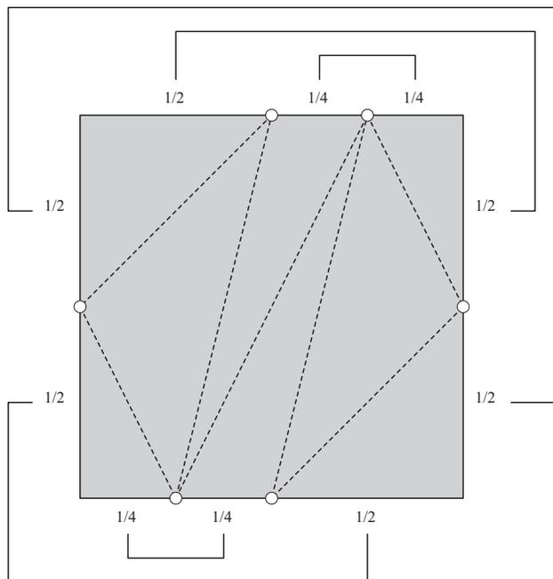
Figure 1: Folding of a unit square produces a polyhedron with 6 vertices (marked) and 8 triangle faces. Lengths of edges on the perimeter are as indicated, and edges connected by an exterior path are identified, i.e., glued to one another.
