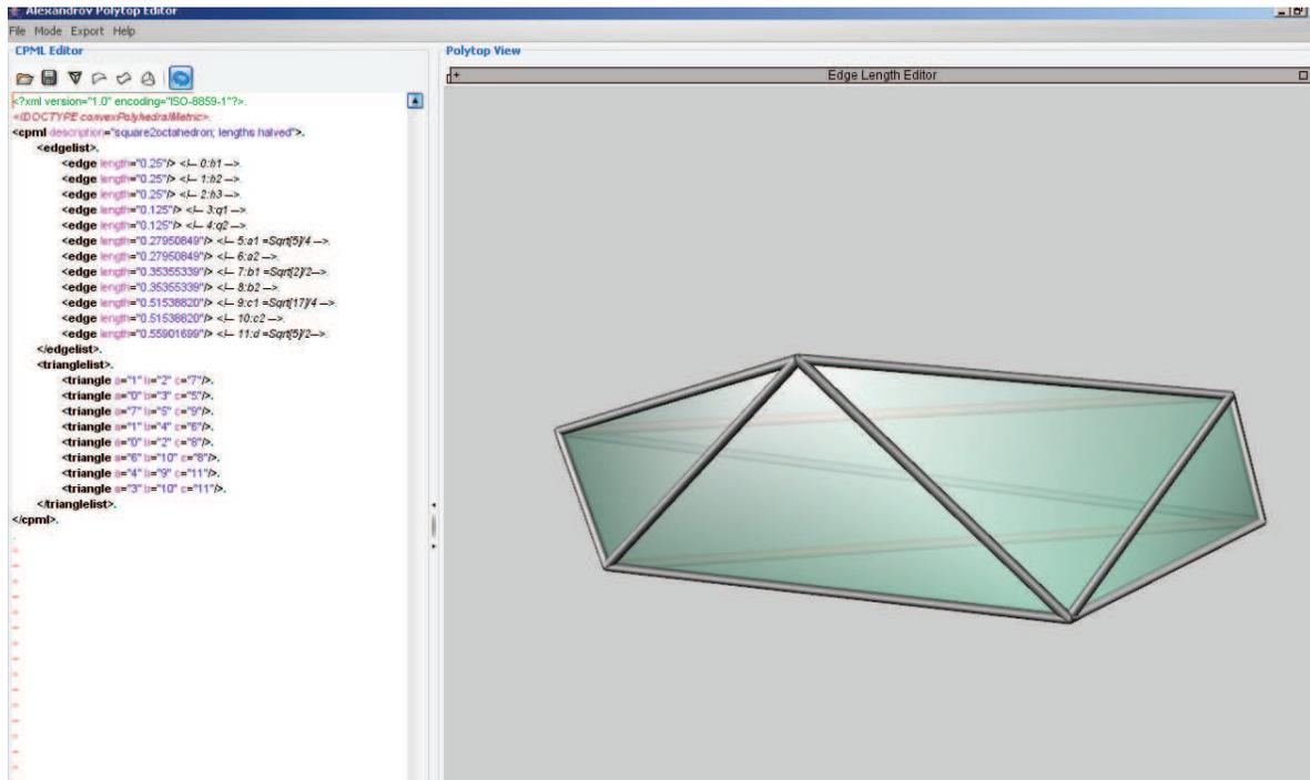
Figure 2: Screen shot of the software. To the left is the XML file describing the triangle gluings, to the right the reconstructed 6-vertex octahedron.
