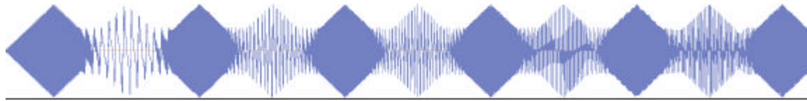
Figure 2. Quicksort grains at beginning of sort. Swapping between right and left sides of list can be readily seen in the jump from high frequency grain to low frequency grain with the difference in frequency diminishing as the middle of the list is neared.
