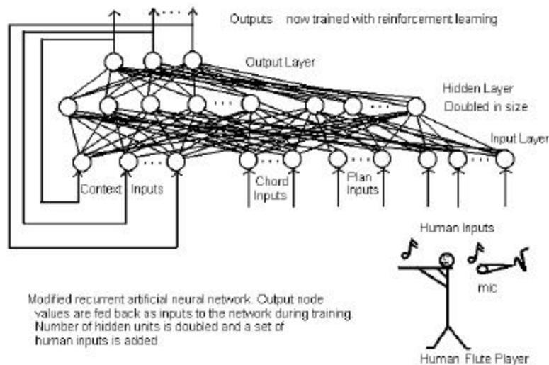
**Figure 5. Experimental network for Phase 2 with reinforcement learning.**
