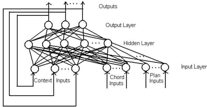
Jordan recurrent artificial neural network. Output node values are fed back as inputs to the network during training.
