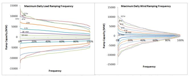
Figure 6 – Maximum daily load and wind ramp frequency for ramps with durations from 10 mintes to 12 hours.
