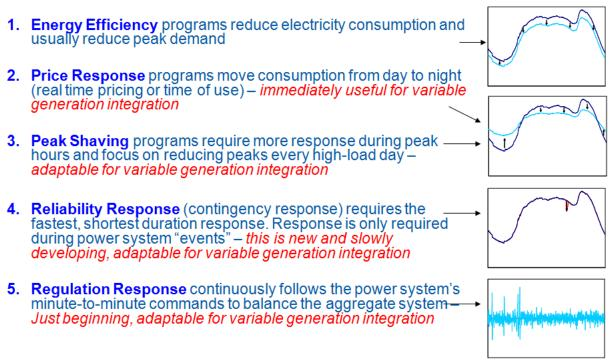
Figure 7 – Four of the five basic types of demand response are potentially useful for facilitating integration of variable renewable generation.
