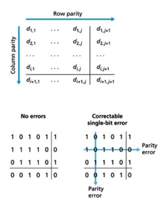
Perhaps the simplest form of error detection is the use of a single parity bit. Suppose that the information to be sent, D has d bits. In an even parity scheme, the sender simply includes one additional bit and chooses its value such that the total number of 1 s in the d + 1 bits (the original information plus a parity bit) is even. For odd parity schemes, the parity bit value is chosen such that there are an odd number of 1s.
