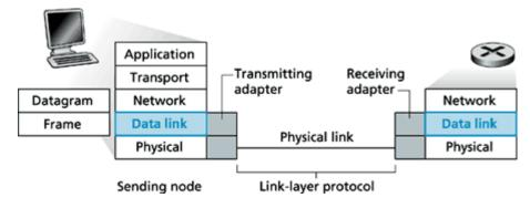
Here, the channel access protocol serves to coordinate the frame transmissions of the many nodes; Frame headers also often include fields for a node's so-called physical address, which is completely distinct from the node's network layer (for example, IP) address.
