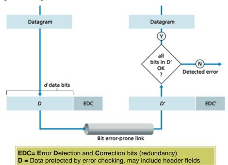
The receiver's challenge is to determine whether or not D' is the same as the original D, given that it has only received D' and EDC'.
