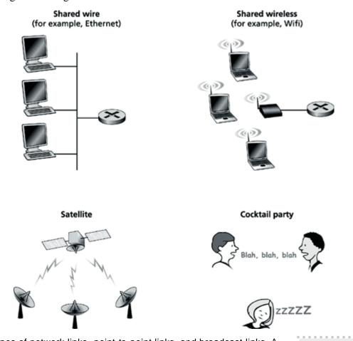
There are two types of network links -point-to-point links, and broadcast links. A point- to-point link consists of a single sender on one end of the link, and a single receiver at the other end of the link. Many link-layer protocols have been designed for point-to-point links;PPP (the point-to-point protocol) and HDLC are two such protocols.
