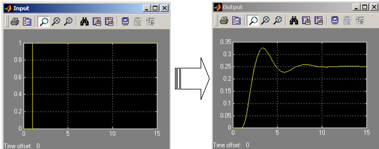
**Fig. 14. Step input and resulting output from second-order system.**
