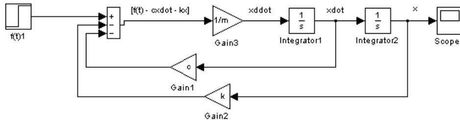
Fig. 10. The finished Simulink model for a SDOF system.
