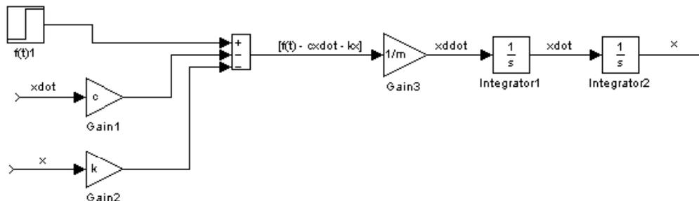
Fig. 9. Integrating the output signal twice.
