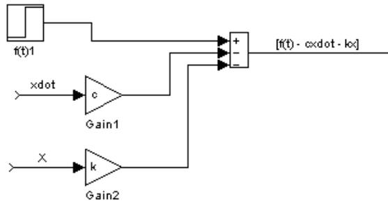
Fig. 7. Summing the input signals.
