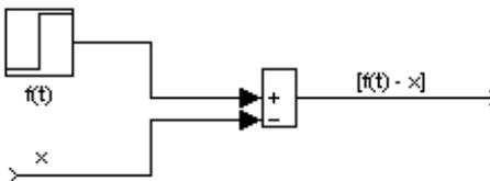
Fig. 2. Summing the input signals.
