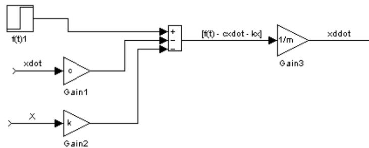
Fig. 8. Applying a gain to the output.
