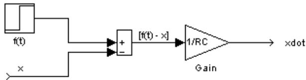
**Fig. 3. Applying a gain to the output.**
