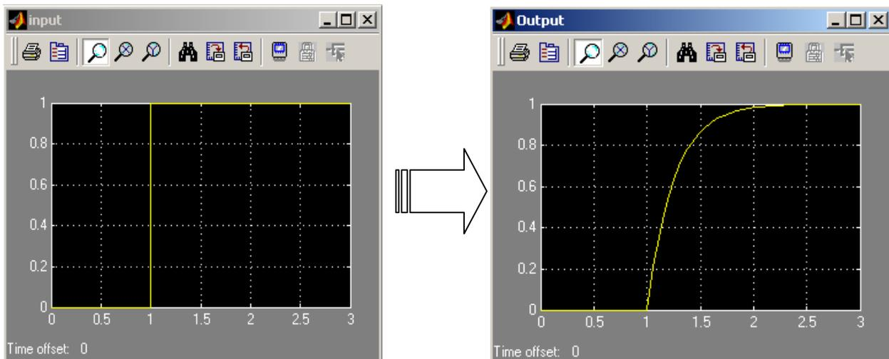
Fig. 13. Step input and resulting output from first-order system.
