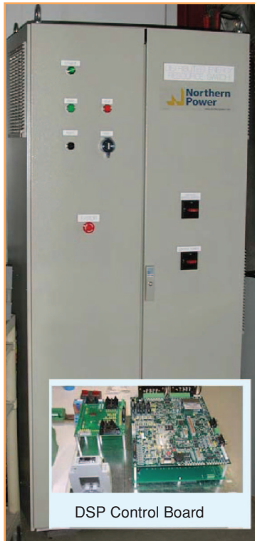
figure 7. Interconnection switch and control board.
