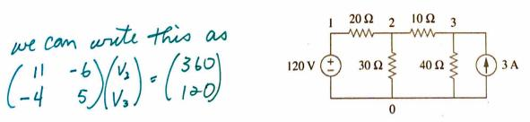
and solve using a computer to find  $\vec{V} = \begin{pmatrix} 81.3 \\ 89.0 \end{pmatrix}$  so  $V_2 = 81.3 V$   $V_3 = 89.0 V$
