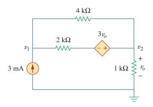
**6)** Using Nodal Analysis, find  $v_0$ . Things to notice about this circuit:
