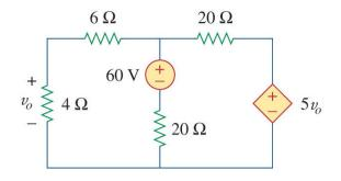
**7)** Using Mesh Analysis, find *v*<sup>o</sup> in the circuit below.
