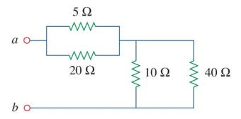
3) Calculate the equivalent resistance,  $R_{ab}$ , at terminals a-b for the circuit below.
