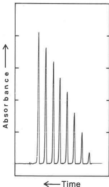
Fig. 2. Absorbance peaks for 1- $\mu$ l samples containing (from right to left) 1, 3, 5, 7, 9, 11, 13, and 15 millimolar (mM) solutions of aluminum in 0.5M HCl. A distilled water sample is shown at the extreme left.
