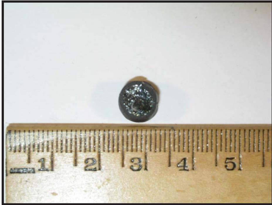
Figure 21: Photo of glass sample inside a graphite crucible, prepared from a sample of Peggy's Cove Monzogranite collected at Cranberry Head
