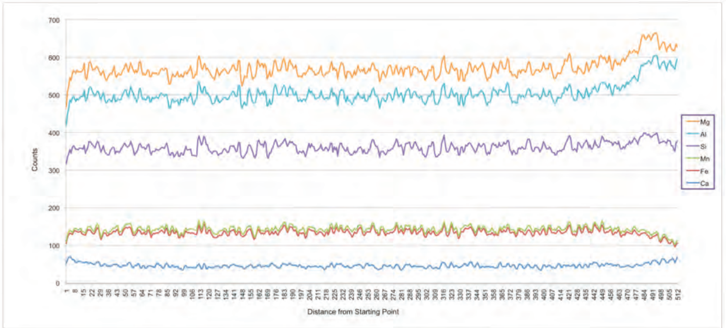
Figure 32. A chemical profile of a large garnet from the dry amphibolite sample of Experiment 6. The garnet is homogenous.
