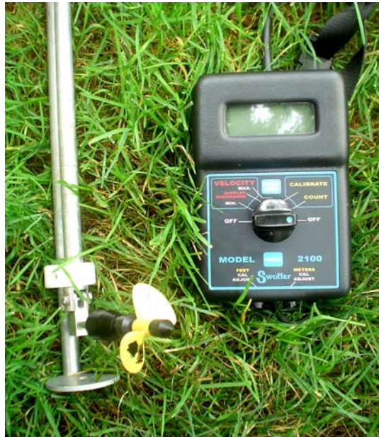
Figure A1. Photo of flowmeter wand and digital meter. The flowmeter consists of a metal rod with marked increments for depth measurement and a propeller for velocity measurement.
