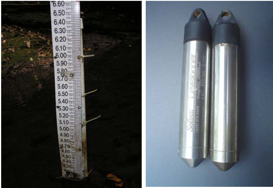
Figure A3. [Left] The water level above an arbitrary point is measured using a staff gage. [Right] Two pressure transducers (levellogger and barologger) installed at QC200. The subtraction of the barologger readings from the levellogger readings yields the water pressure; the latter can be converted to equivalent staff-gage readings by comparing with manual staff-gage measurements.
