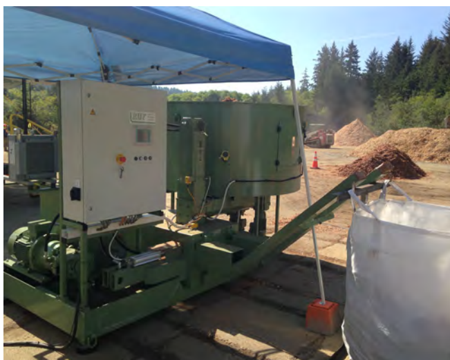
Briquetter and feedstock piles at remote test site.
