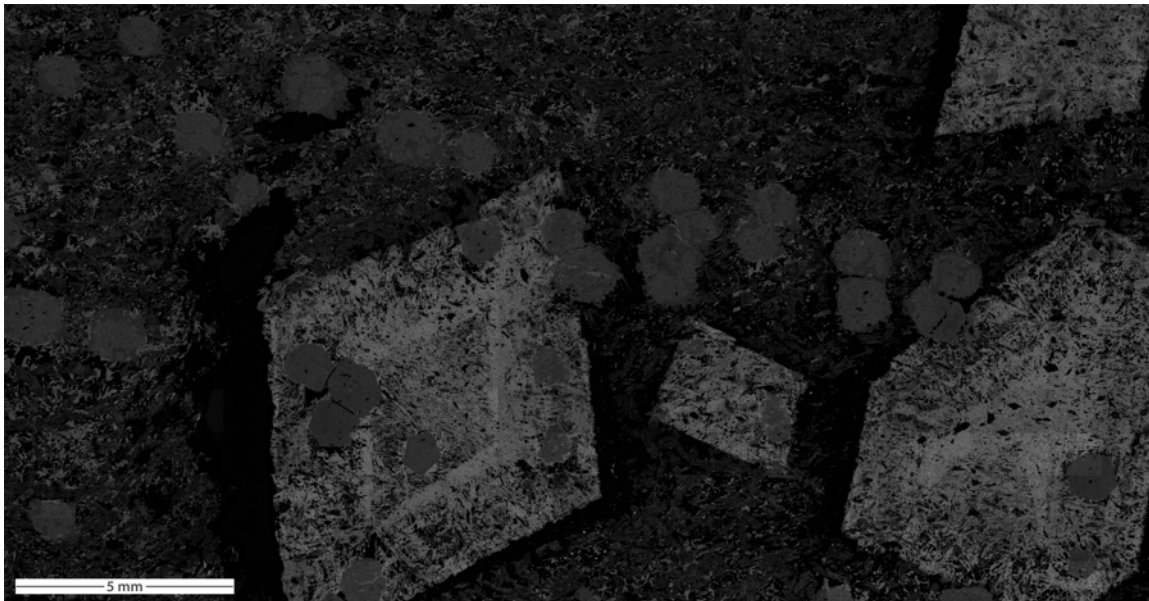
Figure 1 – Thin section phase map (top) and Al-distribution map (bottom) in sample LMA-00-12B. In the top image, note the pseudomorph in the center, which is ~ 1-1.5 cm long, with a calcite-filled pressure shadow around the edges (light yellow), indicating the volume loss resulting from the breakdown of the lawsonite and release of water from the crystal lawsonite structure during breakdown. Ca-rich minerals (epidote-group) are concentrated in the core of the lawsonite whereas the outer part of it is mostly composed of white micas (K- and Na-rich phases) requiring movement of these elements from the matrix into the pseudomorphs during lawsonite-breakdown. In the bottom image, high-Al (light grey) content is concentrated in the diamond shape of the pseudomorphs, retaining its original distribution in the formerly present lawsonite porphyroblasts, indicating that the relative immobility of Al is responsible for the preservation of the lawsonite shape.
