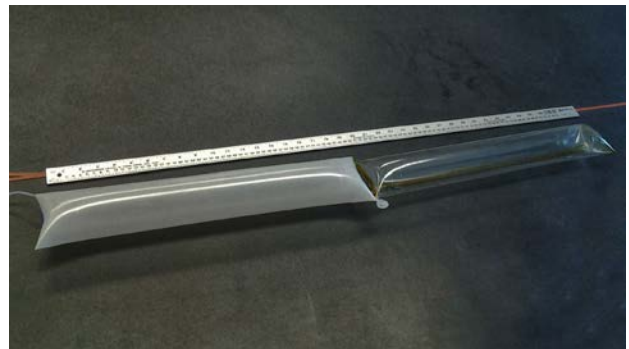
Figure 2: Venus balloon prototype, fully inflated.
