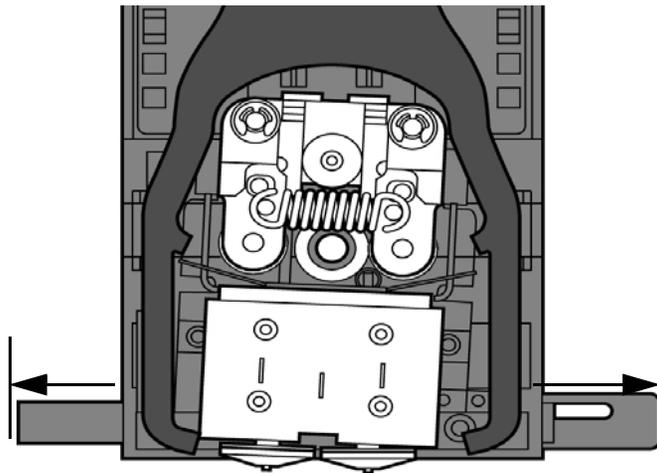
4. Remove any excess material found around the head area.
