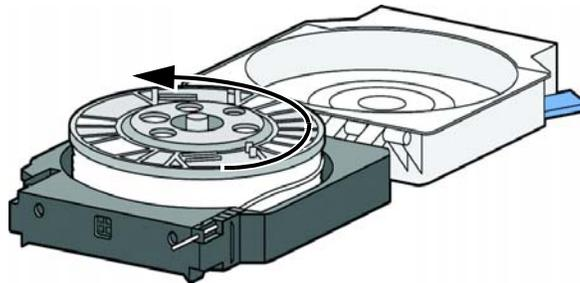
10. Using a cutters, cut the excess 2 inches (50mm) of material from the material guide, leaving a blunt end.
