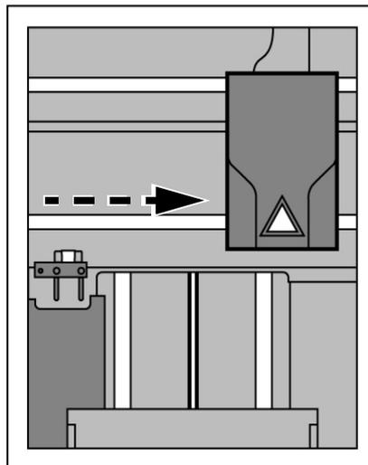
3. Remove the tip wipe assembly by lifting the assembly up and out of the printer. Discard this tip wipe assembly. See [Figure 29](#).
