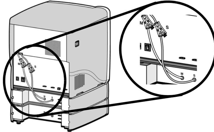
19. Connect the long red striped material tube (M2) from model (M) coupler of lower material bay to **right** side of model Y block by inserting firmly into red couplers. Gently pull the tube to ensure it is properly inserted.
