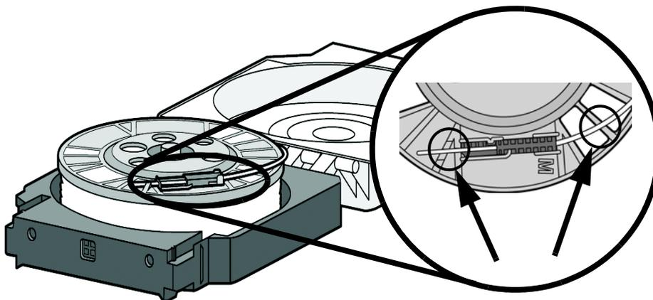
11. Cut the excess material from material guide.
