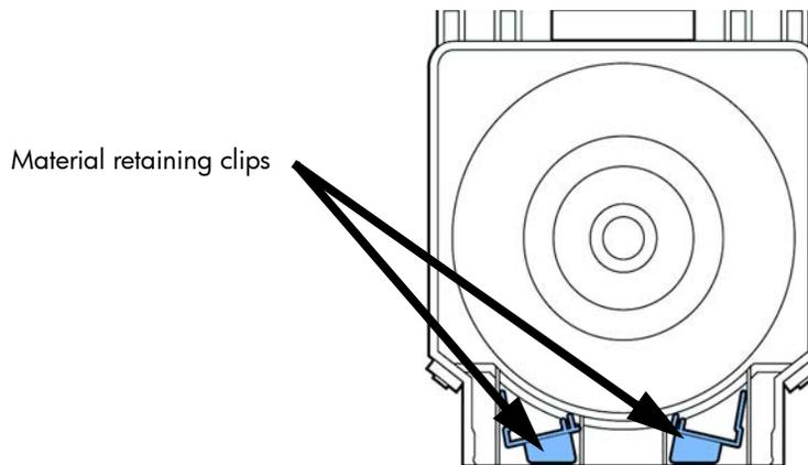
9. Place the material guide in the material guide slot on the spool. See [Figure 24](#).
