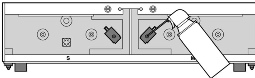
9. Squeeze the spray nozzle for one quick burst (approximately 2 seconds) to clear each Filament Present Switch on the model and support sides of the material bay. If an optional material bay is installed, repeat this procedure for the second bay.
