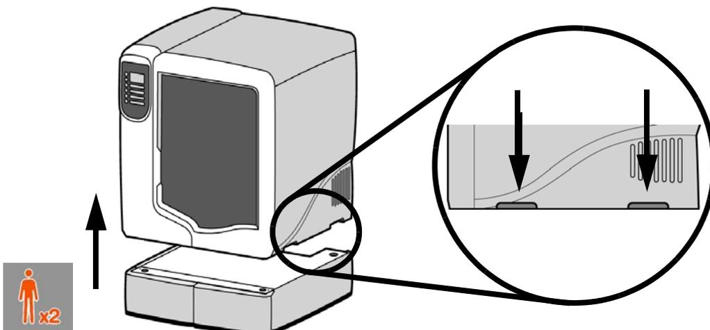
14. Position the second material bay on top of the existing material bay. Be sure the feet and pins are properly aligned. See [Figure 9](#).
