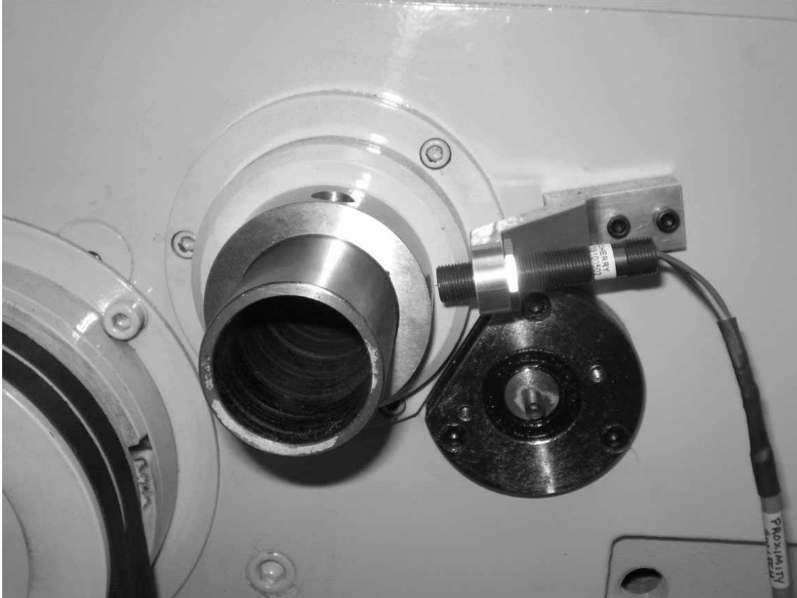
Figure 5-2 1440EX Proximity Sensor
