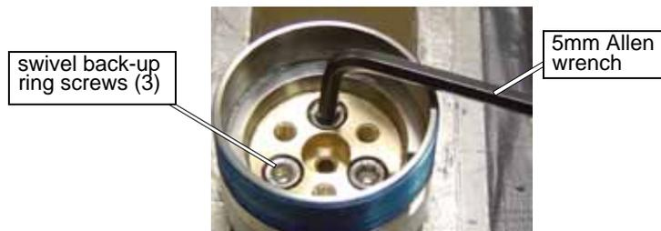
Figure B-12: Tighten the Three Screws to the Swivel Back-up Ring
