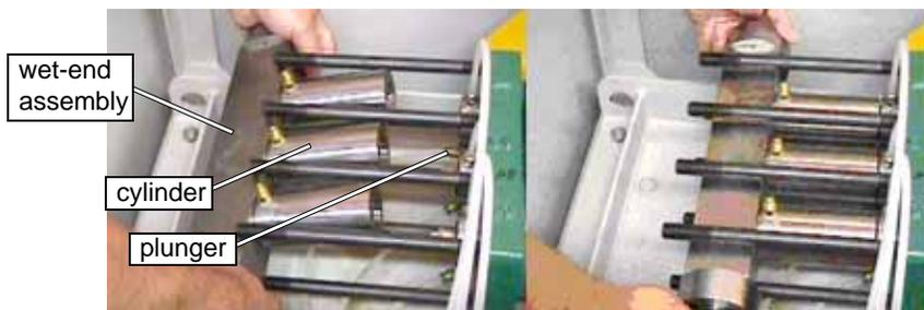
Figure 7-46: Sliding the Wet-end Assembly over the Plungers
