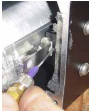
Figure 6-15: Use the Blunt-tip Grease Needle to Lubricate the Four Z-axis Bearings
