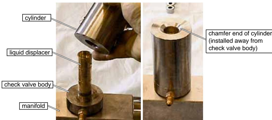
Figure 7-35: Sliding the Cylinder over the Displacer
