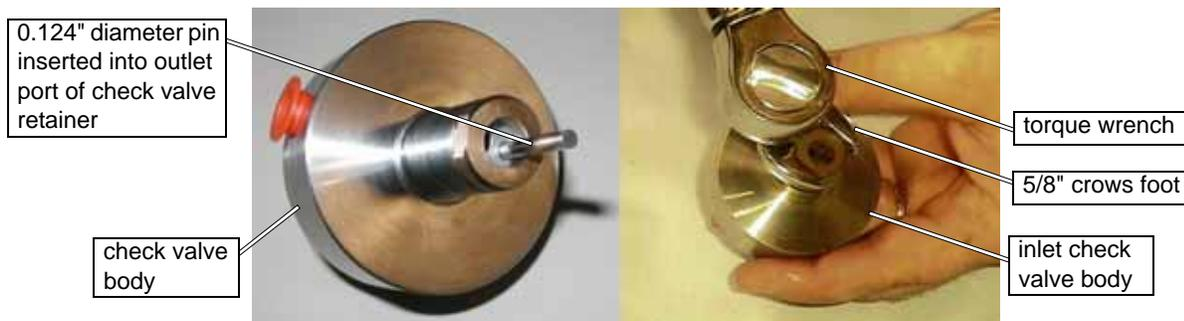
Figure 7-30: Installing the Inlet Retainer Nut
