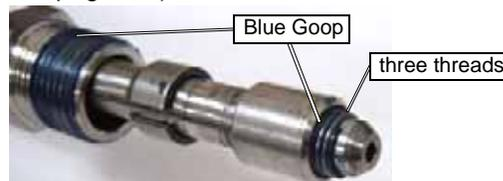
*Figure C-18: Applying Blue Goop and Ensuring Three Threads Show*
