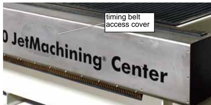
*Figure 6-8: Remove Cover Plate to Access the 80160 X-axis Timing Belt*
