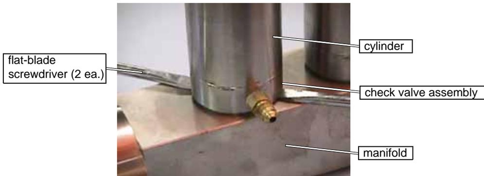
Figure 7-8: Removing the Cylinder and Check Valve Assembly
