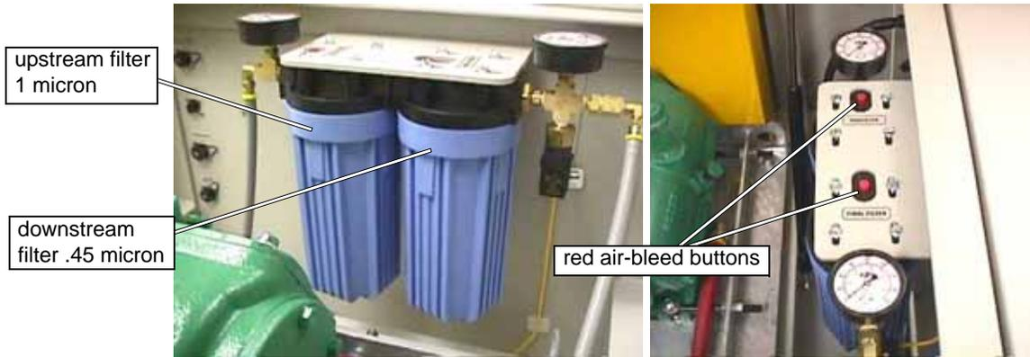
Figure 7-52: Low-pressure Water Filters with Pressure Gauges
