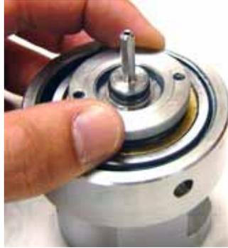
*Figure B-22: Hand Tighten the Bearing Lock Nut*
