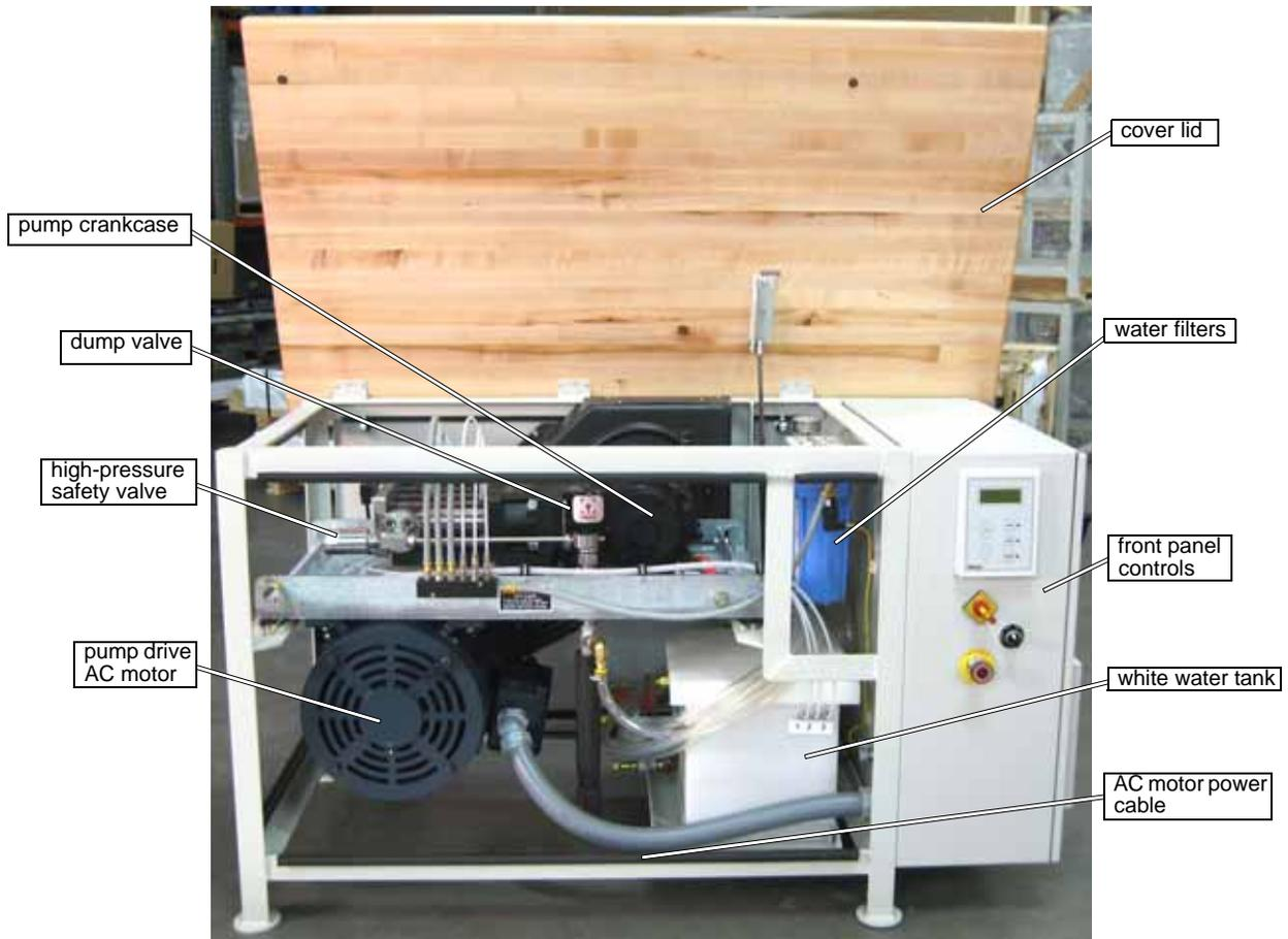
Figure 3-3: Pump with Top Lid Open and Front Panel Removed
