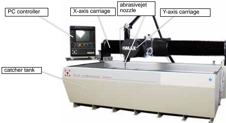
Figure 2-9: Components of the JetMachining Center Models 2626, 2626xp, 2652, 5555, and 55100 (55100 illustrated)
