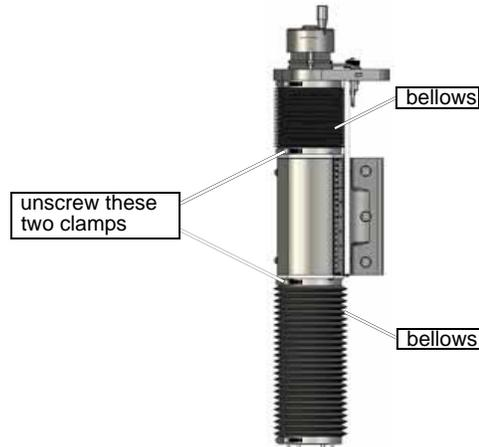
Figure 6-12: Z-axis Assembly
