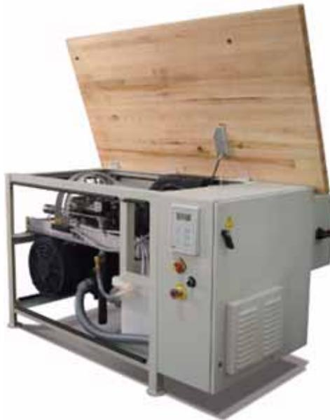
*Figure 3-1: OMAX High-Pressure Water Pump*
