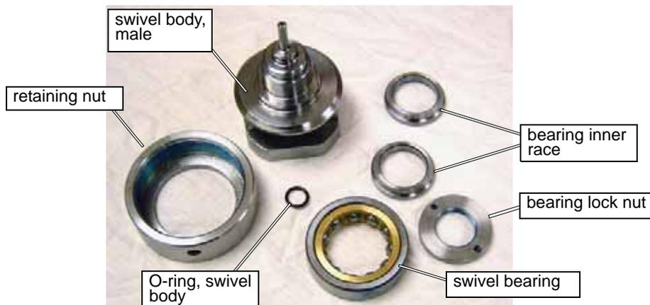
*Figure B-17: Male Swivel Body Bearing Components*
