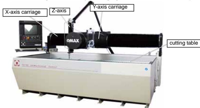
*Figure 2-18: X-Y Carriage Components of the JetMachining Center Models 2626, 2626|xp, 2652, 5555, and 55100 (55100 illustrated)*
