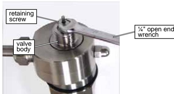
Figure C-3: Removing the Retaining Screw from the Valve Body
