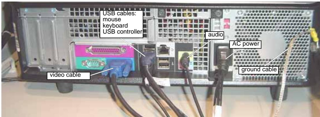
Figure 2-17: PC Rear Panel Cable Connections
