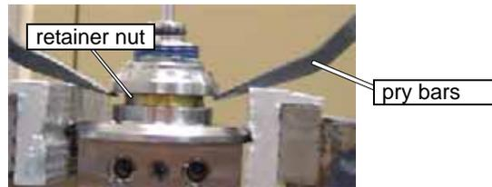
*Figure B-16: Use Pry Bars to Remove the Inner Race from the Swivel Body*
