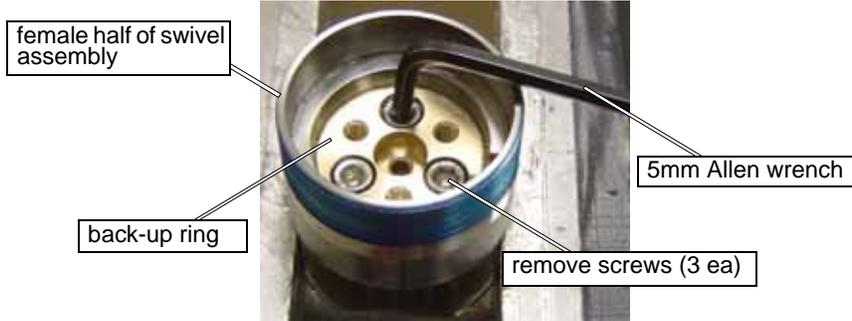
Figure B-7: Remove the Three Swivel Assembly Screws with the 5mm Allen Wrench
