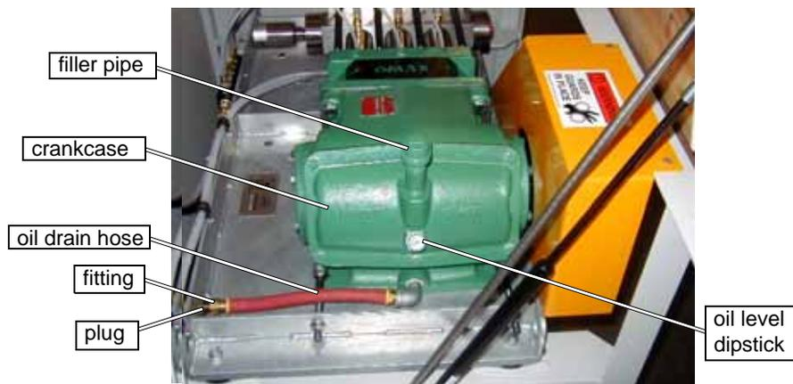
Figure 7-54: Pump Crankcase, Oil Drain Hose, Filler Pipe
