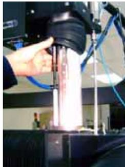
Figure 6-13: Lift Bellows to Expose Grease Points
