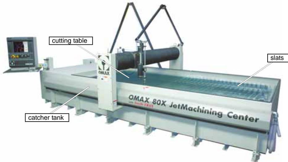
Figure 2-25: JetMachining Center Catcher Tank
