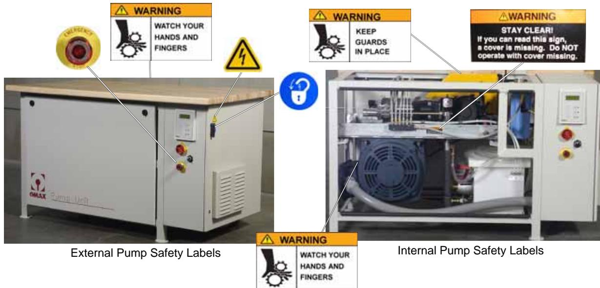
Figure 1-5: Safety Labels OMAX Pumps
