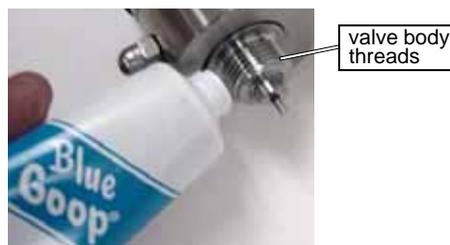
*Figure C-19: Applying Blue Goop to the Valve Body Threads*
