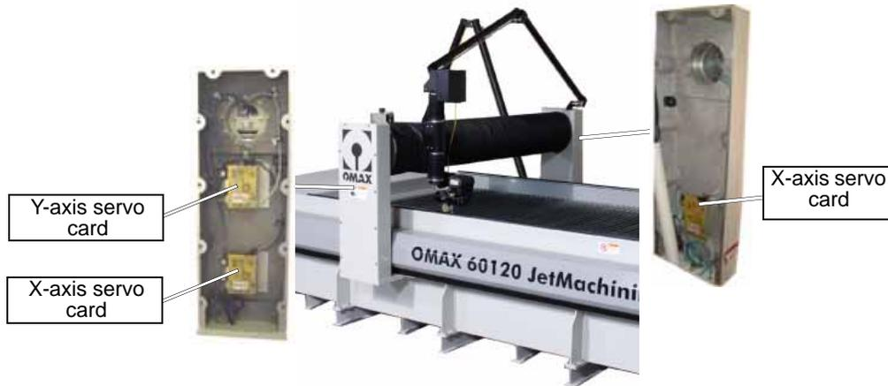
Figure 4-5: Servo Card Locations for Y and X-axis for Bridge-style Tables
