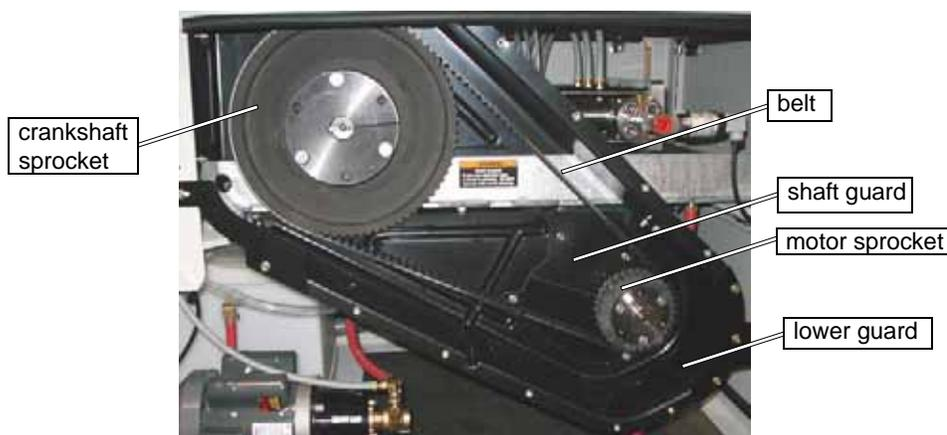
*Figure 7-56: OMAX Pump Belt with Belt Guard Cover Removed*
