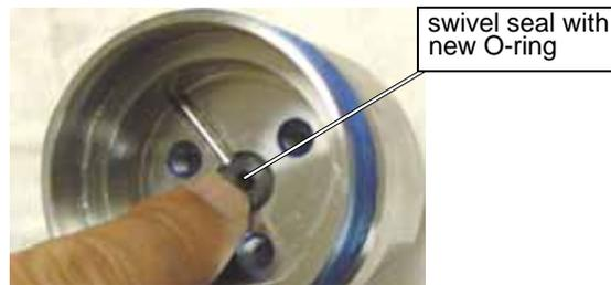
Figure B-10: Insert the Swivel Seal with New O-ring into the Swivel Body
