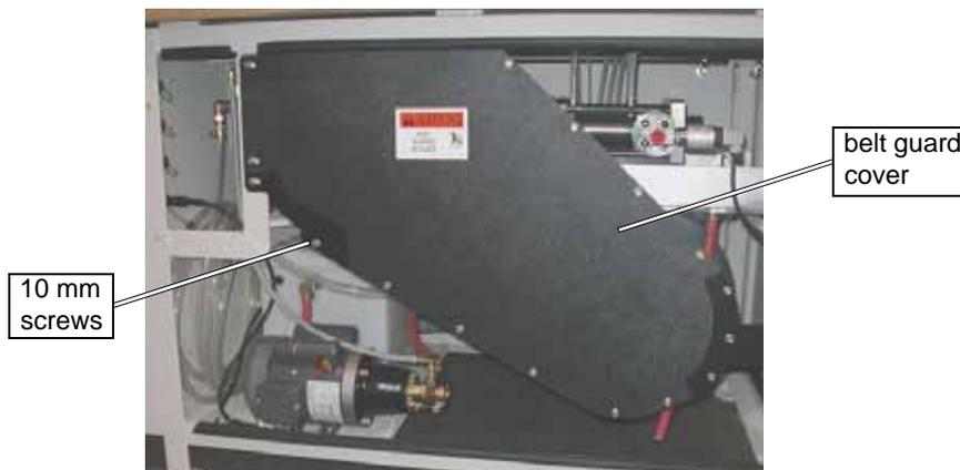
*Figure 7-55: OMAX Pump Belt Guard Cover*
