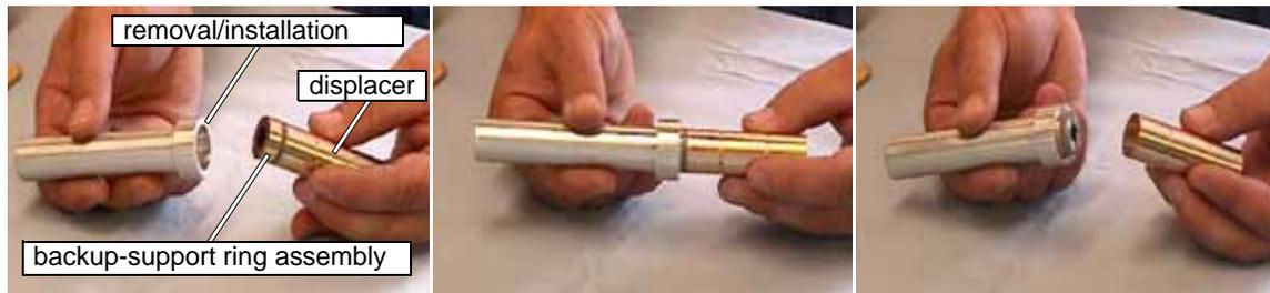
Figure 7-12: Separating the Backup-Support Ring Assembly from the Displacer.
