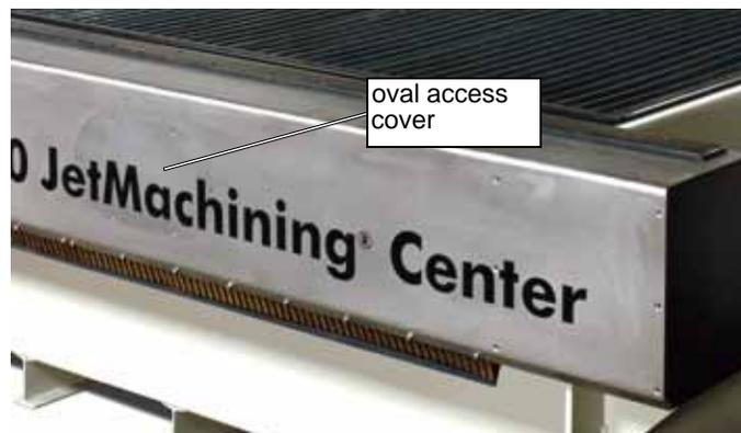
Figure 6-17: Remove 80160 Access Covers to Reach Rail Lubrication Points
