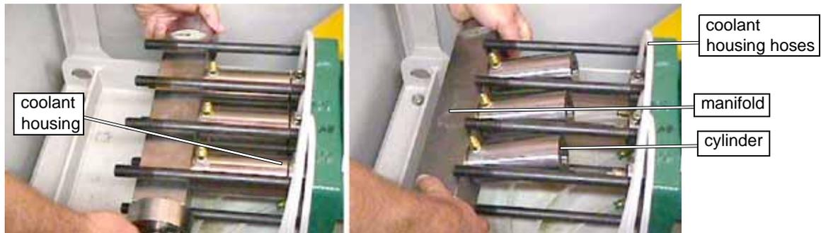
Figure 7-5: Removing the Wet-end Assembly
