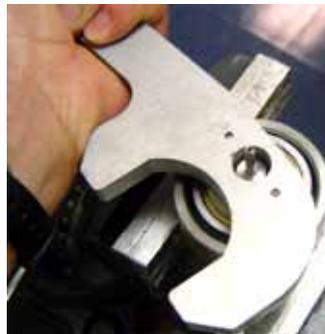
*Figure B-23: Fully Tighten the Bearing Lock Nut using the Swivel Spanner Wrench*
