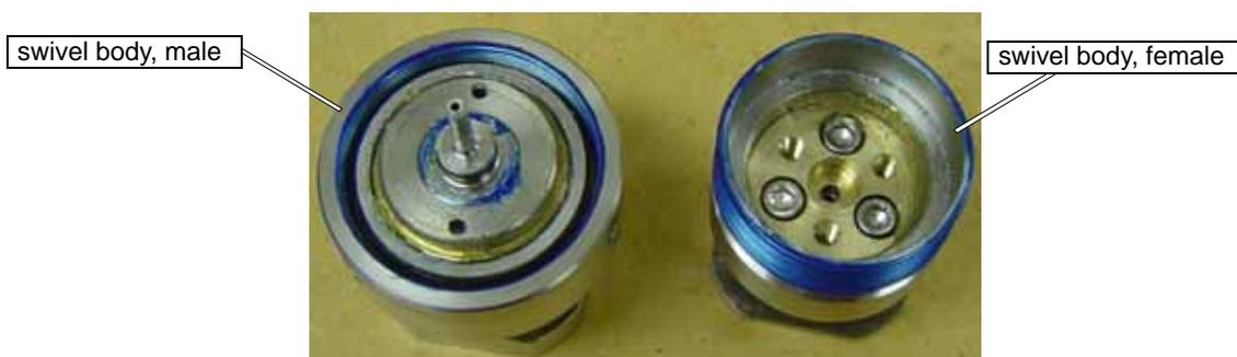
Figure B-6: Separate the Swivel Assembly into its Male and Female Halves
