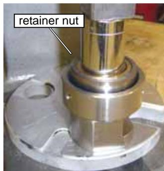
*Figure B-20: Installing the Bearing Assembly with the Arbor Press*
