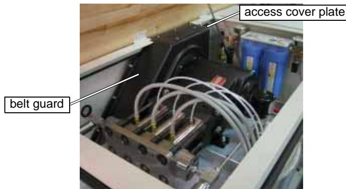
Figure 7-39: Access Cover Plate on Top of Pump Belt Guard
