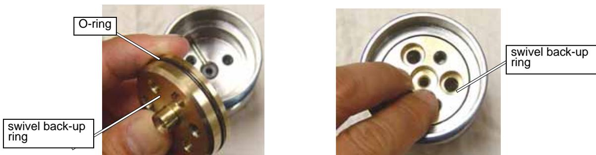
Figure B-11: Insert the Swivel Back-up Ring with a New O-ring Installed into the Swivel Body
