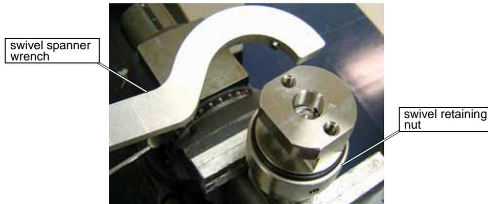
Figure B-5: Use the Swivel Spanner Wrench to Unscrew the Swivel Retaining Nut
