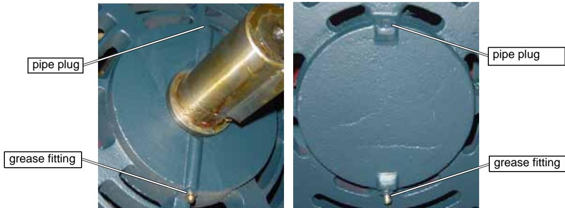
Figure 7-57: Location of Front and Rear Motor Grease Fittings and Pipe Plugs
