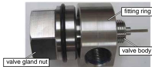
Figure C-16: Sliding the Valve Gland Nut and Fitting Ring onto the Valve Body
