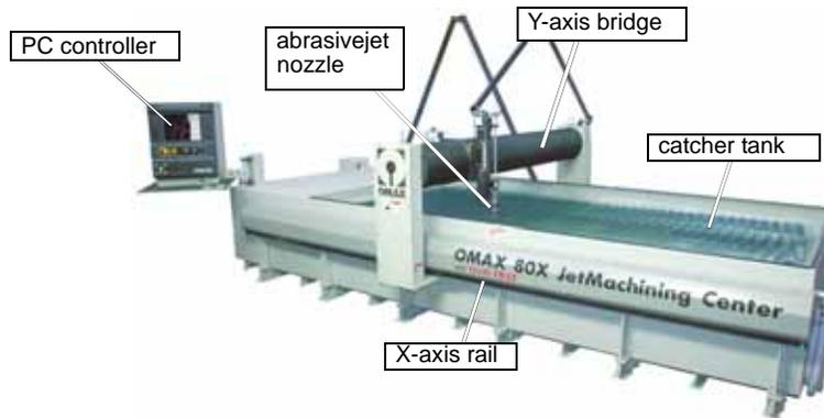
Figure 2-10: Components of the JetMachining Center Models 60120, 80160, and 80X (80X illustrated)
