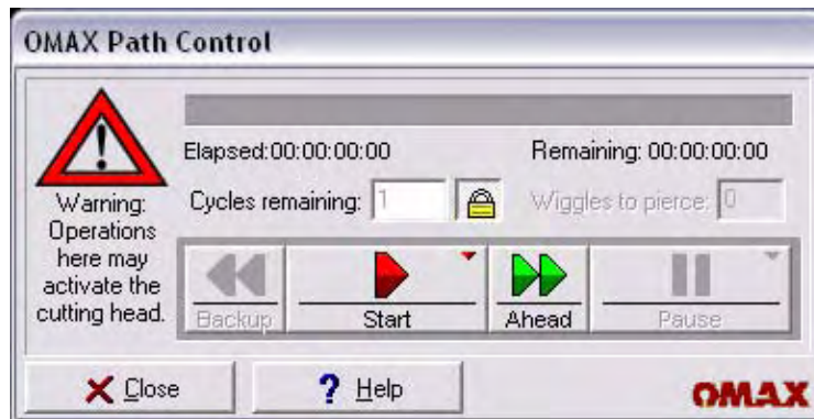
Figure 4-81: Click Start to Pressurize the Adjustable Dump Orifice
