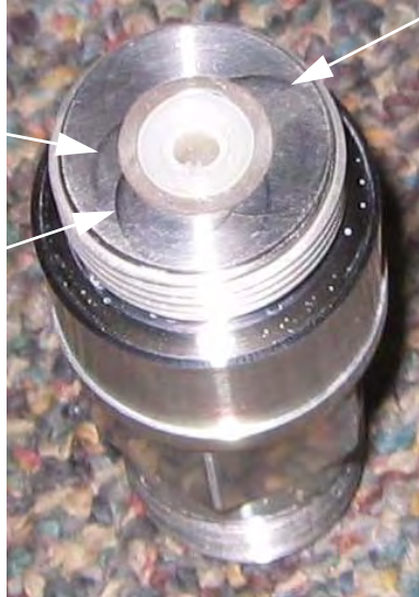
Figure 4-32: Damage Caused by an Off-center Orifice
