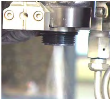
Figure 4-21: Purging the High-pressure System of Contaminates with the Nozzle Removed
