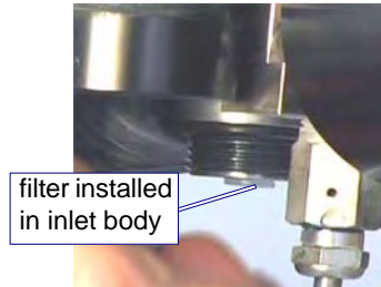
Figure 4-23: Filter Seal Assembly Inserted into Inlet Body
