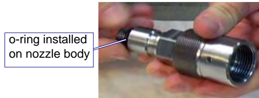
Figure 4-26: Installing the O-ring on the Nozzle Body
