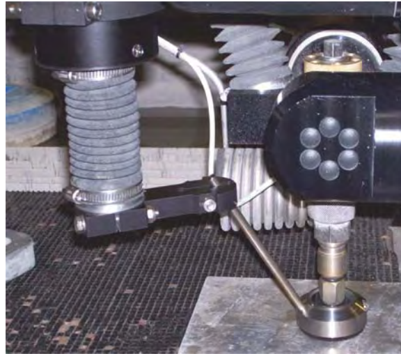
Figure 2-21: OMAX Terrain Follower Attached to a Tilt-A-Jet
