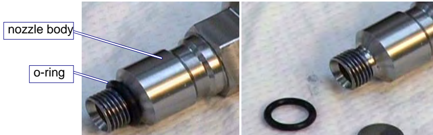
Figure 4-9: Removing the O-ring from the Nozzle Body
