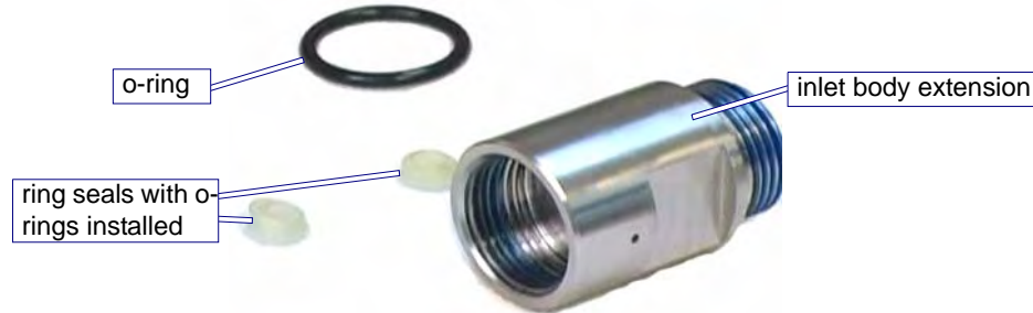
Figure 4-63: Removing O-ring and Ring Seals from the Inlet Body Extension
