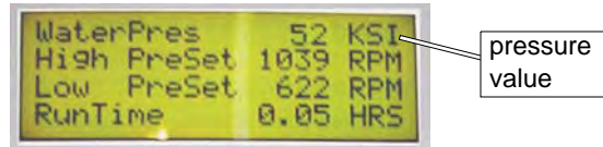
Figure 4-79: Set the KSI for WaterPres on the Pump's LCD
