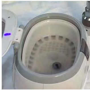
Figure 4-11: Cleaning Parts in Ultrasonic Cleaner with White Vinegar
