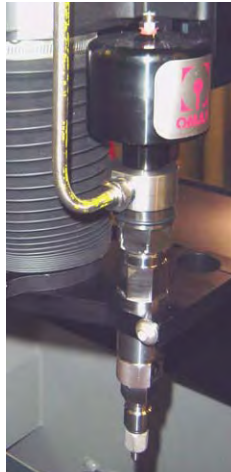
Figure 4-72: Dual On/Off Valve with MAXJET®5 Nozzle
