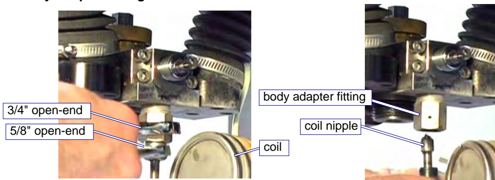
Figure 4-41: Removing the Coil Nipple From the On/Off Valve Body Adapter Fitting
