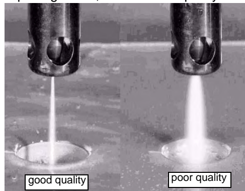
Figure 3-13: Example of Both Good and Poor Quality Jet Streams
