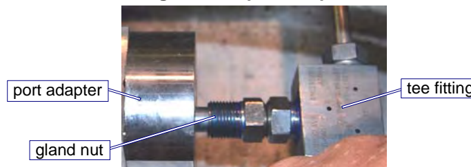
Figure 4-86: Removing the Gland Nut and Tubing from the Port Adapter
