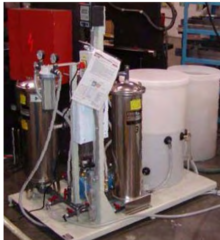
Figure 2-20: Closed Loop Water Recycling System
