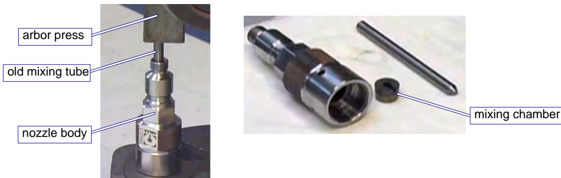
Figure 4-8: Pressing the Mixing Chamber from the Nozzle Body
