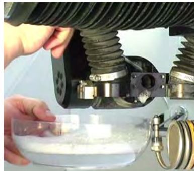
Figure 4-50: Cleaning the Inlet Body Hole with Brush and Soapy Water
