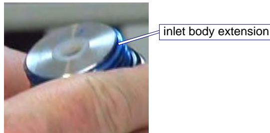
Figure 4-61: Inspecting the Body Extension for Erosion Marks
