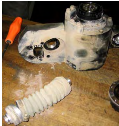
Figure 4-38: Abrasive Damage from Not Using a Nozzle Muff
