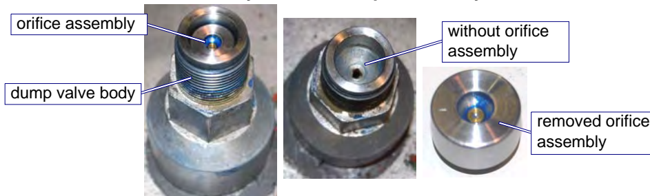
Figure 4-90: Removing the Orifice Assembly from the Dump Valve Body
