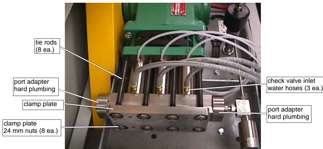
Figure 5-2: High-pressure Wet End Assembly
