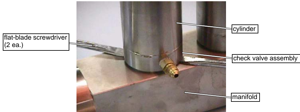
Figure 5-8: Removing the Cylinder and Check Valve Assembly
