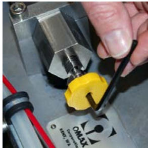
Figure 4-11: Using a 3/16" Allen Wrench to Adjust the ADO Pressure
