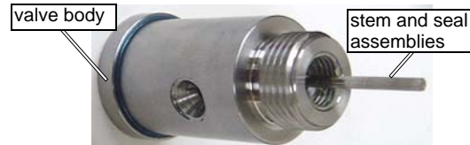
Figure 6-101: Insert the Stem and Seal Assemblies into the Valve Body
