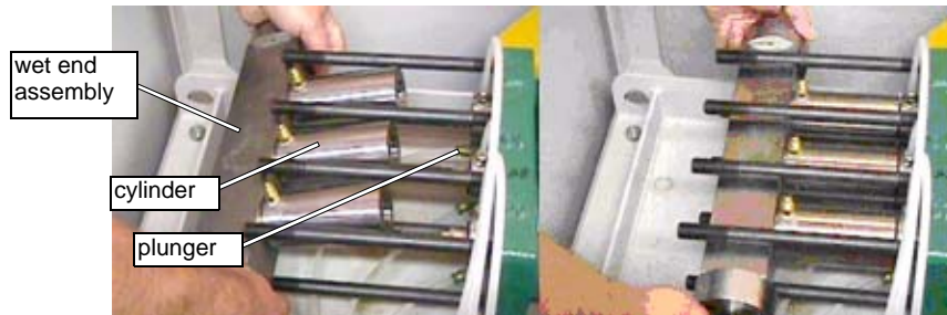
Figure 5-46: Sliding the Wet End Assembly over the Plungers
