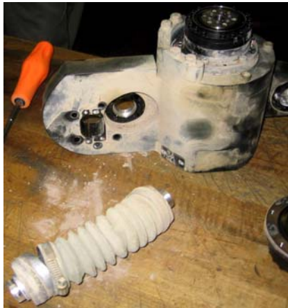
Figure 6-60: Abrasive Damage from Not Using a Nozzle Muff
