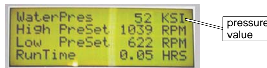
Figure 4-8: Set the KSI for WaterPres on the Pump's LCD
