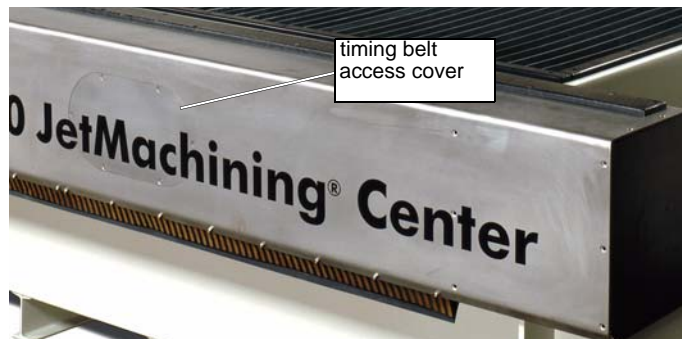
Figure 6-10: Remove Cover Plate to Access the 80160 X-axis Timing Belt
