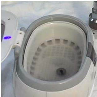
Figure 6-33: Cleaning Parts in Ultrasonic Cleaner with White Vinegar
