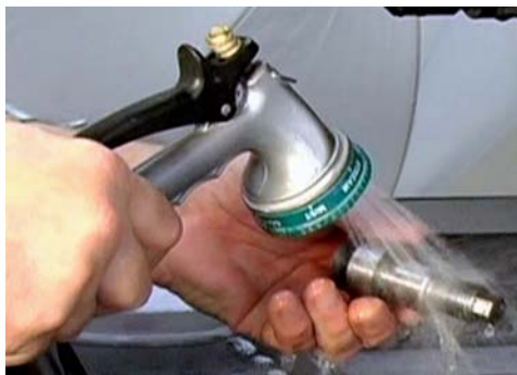
Figure 6-32: Rinsing Parts with Clean Water
