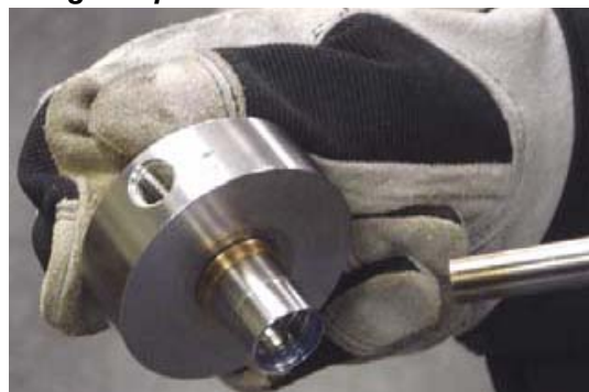
Figure 5-21: Using a Propane Torch to Remove the Support Ring
