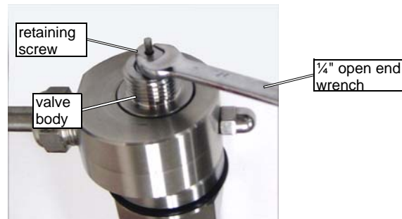
Figure 6-91: Removing the Retaining Screw from the Valve Body
