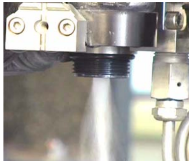
Figure 6-43: Purging the High-pressure System of Contaminates with the Nozzle Removed
