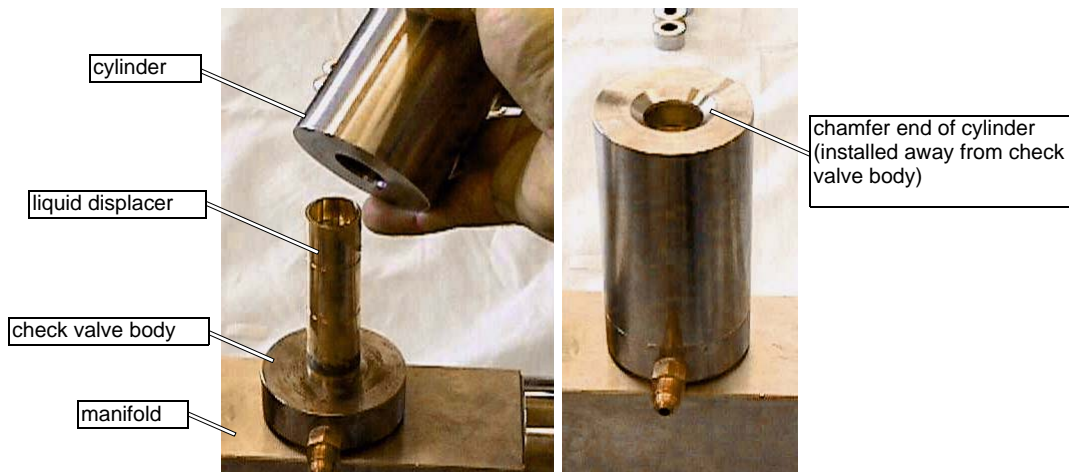
Figure 5-35: Sliding the Cylinder over the Displacer
