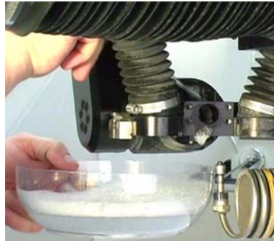
Figure 6-67: Cleaning the Inlet Body Hole with Brush and Soapy Water
