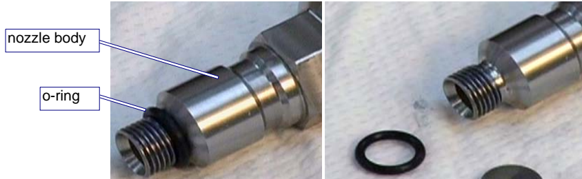
Figure 6-31: Removing the O-ring from the Nozzle Body
