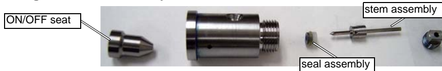
Figure 6-98: Discard the ON/OFF Seat, Seal Assembly, and Stem Assembly
