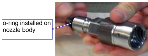
Figure 6-48: Installing the O-ring on the Nozzle Body
