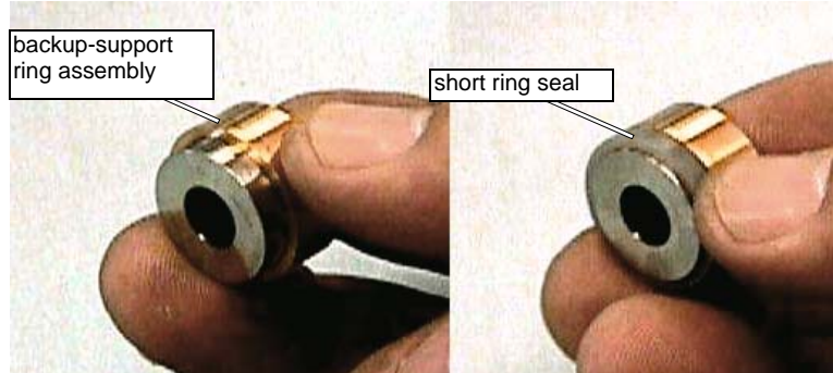
Figure 5-43: Installing the Short Ring Seal onto the Backup-Support Ring Assembly
