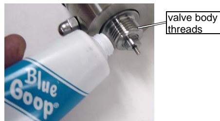
Figure 6-107: Applying Blue Goop to the Valve Body Threads
