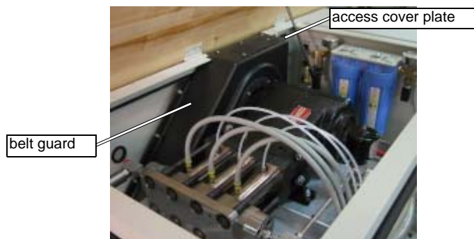
Figure 5-39: Access Cover Plate on Top of Pump Belt Guard
