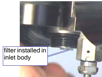
Figure 6-45: Filter Seal Assembly Inserted into Inlet Body
