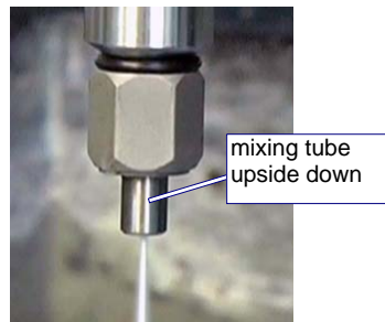
Figure 6-41: Installing the Mixing Tube Upside Down to Dislodge a Clogged Opening
