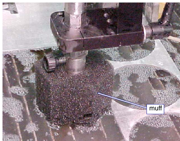
Figure 4-33: Cutting Nozzle with a Muff Attached
