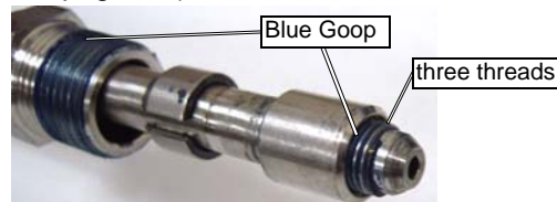
Figure 6-106: Applying Blue Goop and Ensuring Three Threads Show
