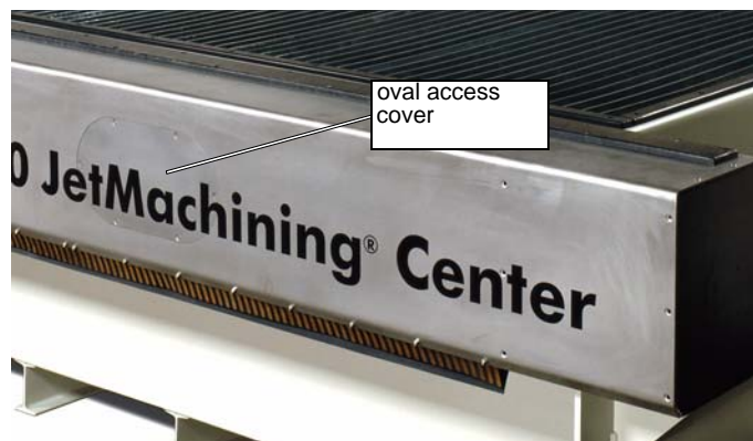
Figure 6-19: Remove 80160 Access Covers to Reach Rail Lubrication Points
