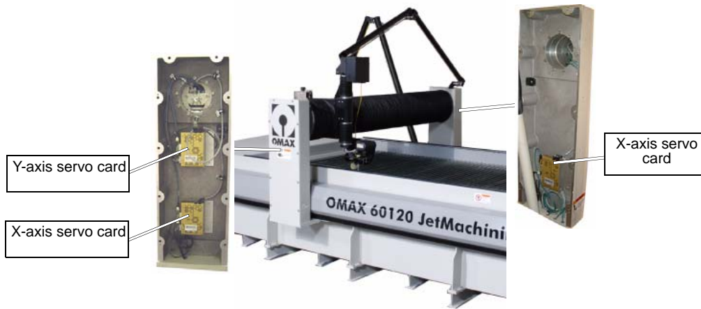
Figure 7-1: Servo Card Locations for Y and X-axis for Bridge-style Table
