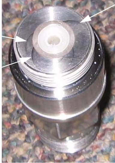
Figure 6-54: Damage Caused by an Off-center Orifice
