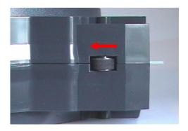
Figure 11: Direction to move cartridge roller
