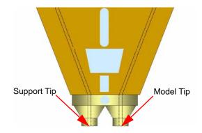
Figure 13: Close-up of extrusion tips
