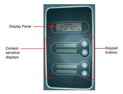
Figure 9: Dimension display panel and keypad
