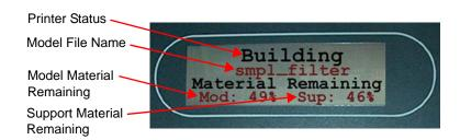
Figure 15: Display panel during build
