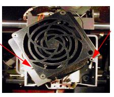
Right Side Mounting Screw in Retaining Notch
