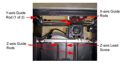
Figure 17: Lead Screw and Guide Rod Identification
