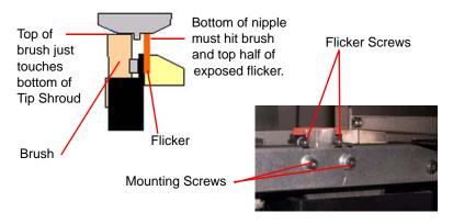
Figure 16: Replacing the tip cleaning brush
