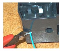
Figure 12: Snipping the material filament
