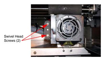
Figure 20: Location of swivel head screws (2) (Head shown is SST - Screw location is the same for BST)
