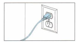
Figure 5: Connecting to a grounded electrical outlet
