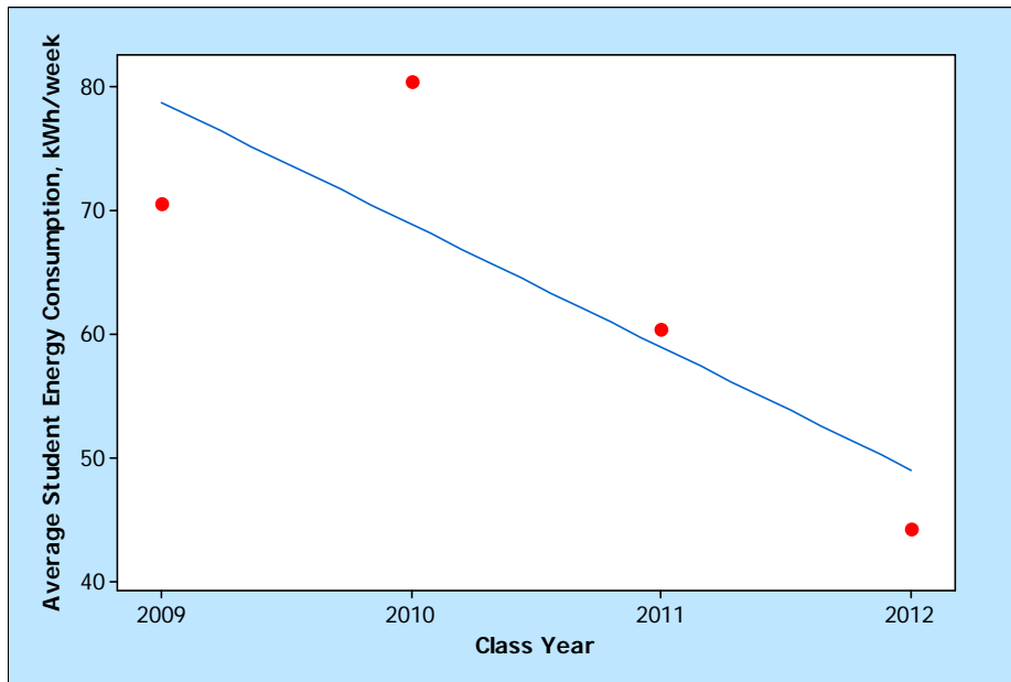
Figure 4. Linear regression of class year versus per capita energy consumption. The equation of the regression is E = 19972 - 9.902 * Y where E is per capita or average energy consumption and Y is class year. R^2 = 68.6 , F = 4.36 , and p = 0.172 .
