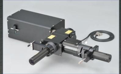
Automatically adjusts the focus and incident angle of the laser for TIRF observation.
