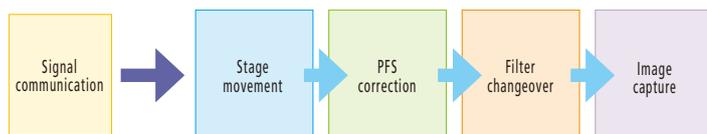
Once it receives command signals from a PC, the Ti controller takes over control of each motorized component, allowing the communication time between PC and each motorized component to be eliminated, minimizing overall operation time.
