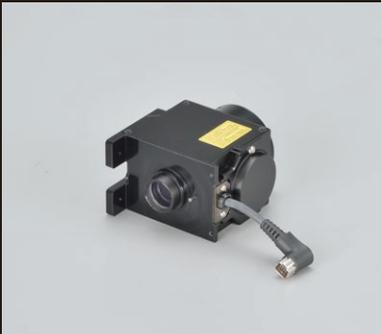
Enables two optical paths to be added and makes motorized path switching possible
