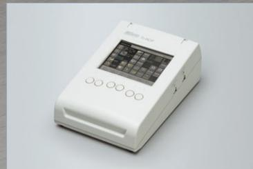
Microscope status can be confirmed with icons. The microscope can be operated via the touch panel.
