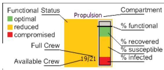
Figure 4. The visualization of the propulsion compartment in SDDT
